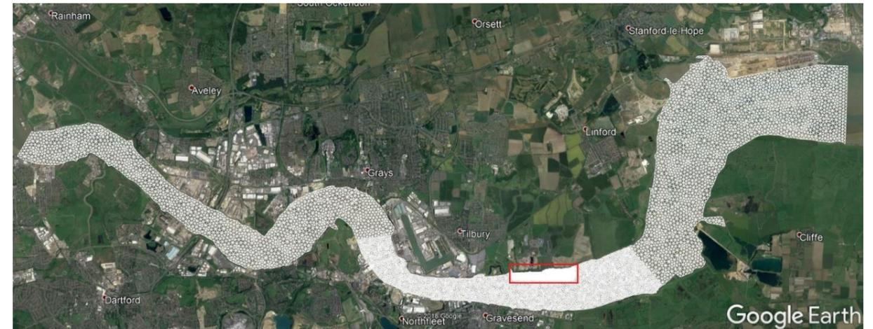
Figure 2.1: Extent and resolution of model grid.
