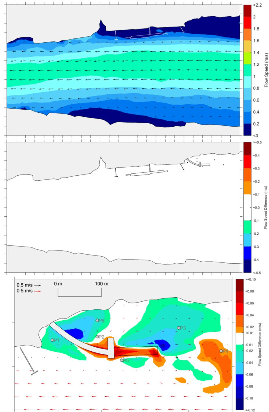
Figure 3.8: Baseline flow speeds during flood tide (top). Effect of AIL Facility with RoRo vessel on baseline flows (middle and bottom).
