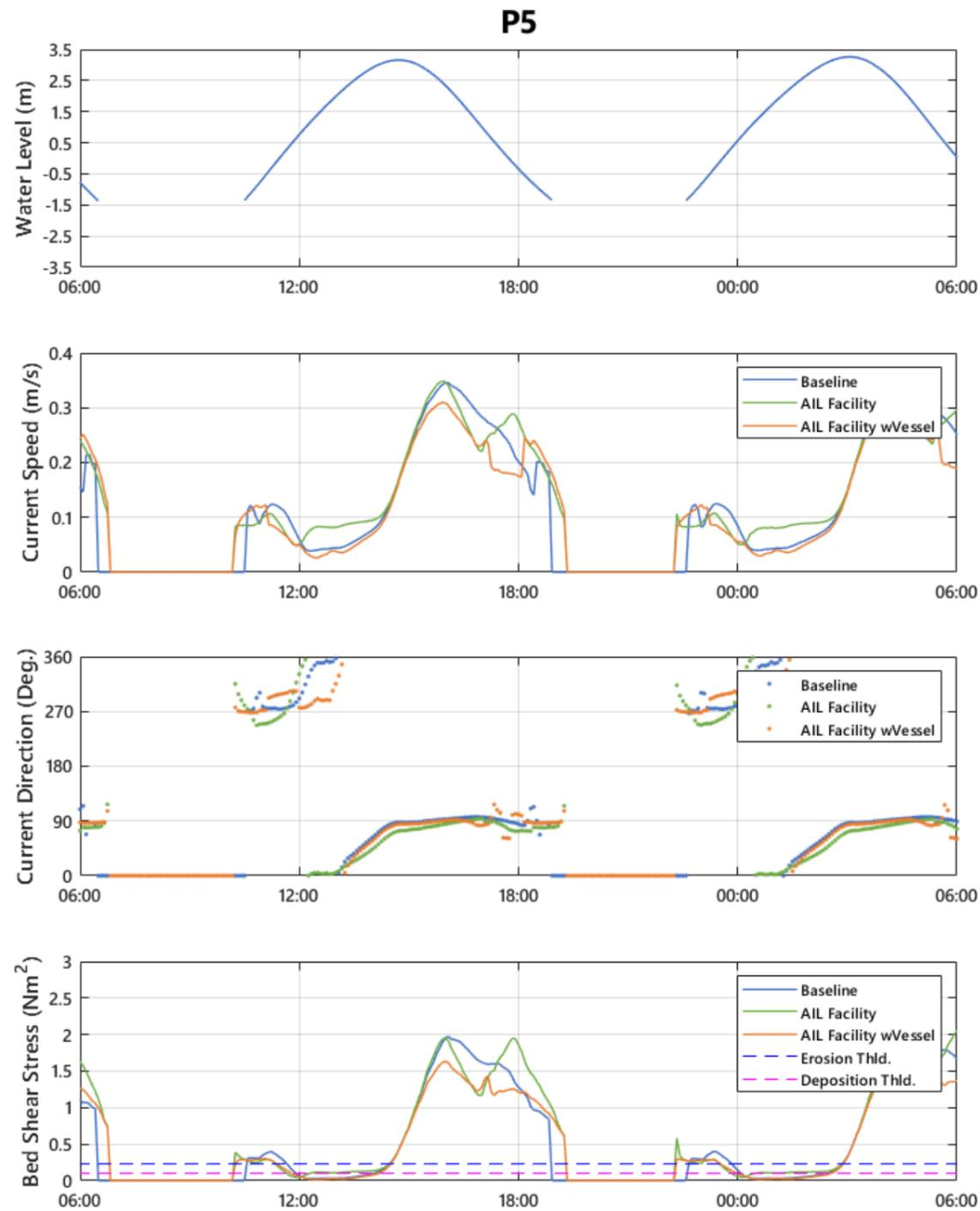
Figure 3.7: Comparison of current speed, direction and BSS as a result of the AIL Facility and AIL Facility with RoRo vessel compared to the baseline at P5.
