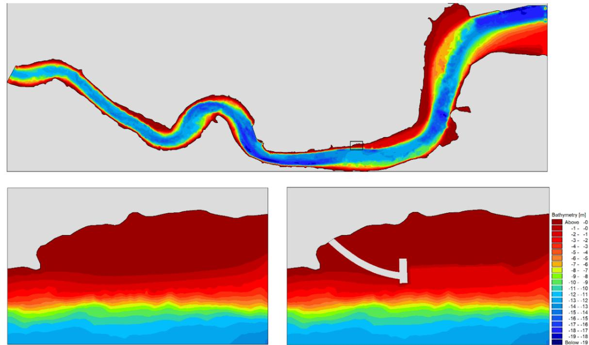
Figure 2.2: Interpolated bathymetry over the whole model domain (top) and across the site (bottom left). Bottom right shows the mesh bathymetry as a result of the addition of the AIL Facility.
