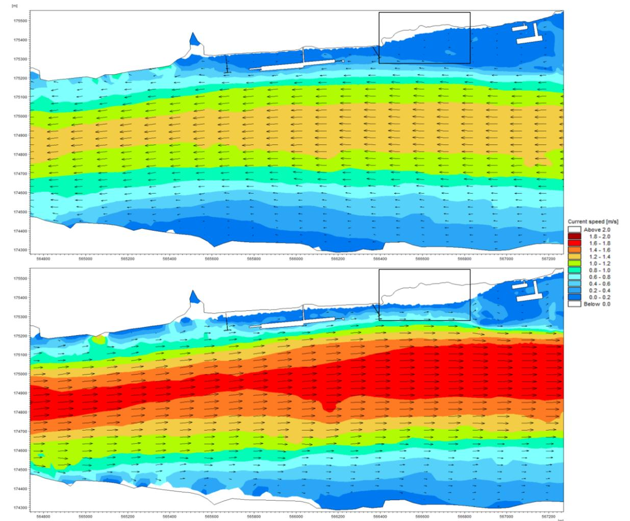
Figure 2.8: Local flow speeds during peak flood (top) and peak ebb (bottom). Black box indicates the site.
