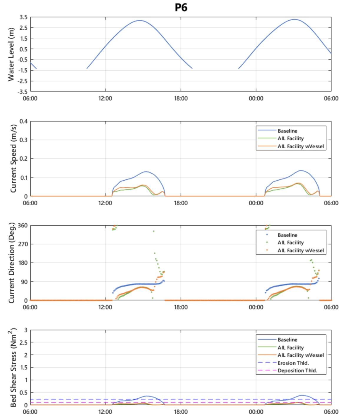
Figure 3.5: Comparison of current speed, direction and BSS as a result of the AIL Facility and AIL Facility with RoRo vessel compared to the baseline at P6.
