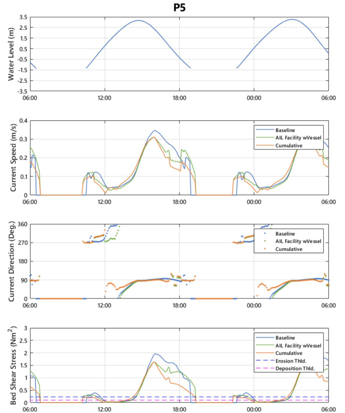
Figure 3.14: Comparison of current speed, direction and BSS as a result of the AIL Facility with RoRo vessel, and Cumulative scenario compared to the baseline at P5.
