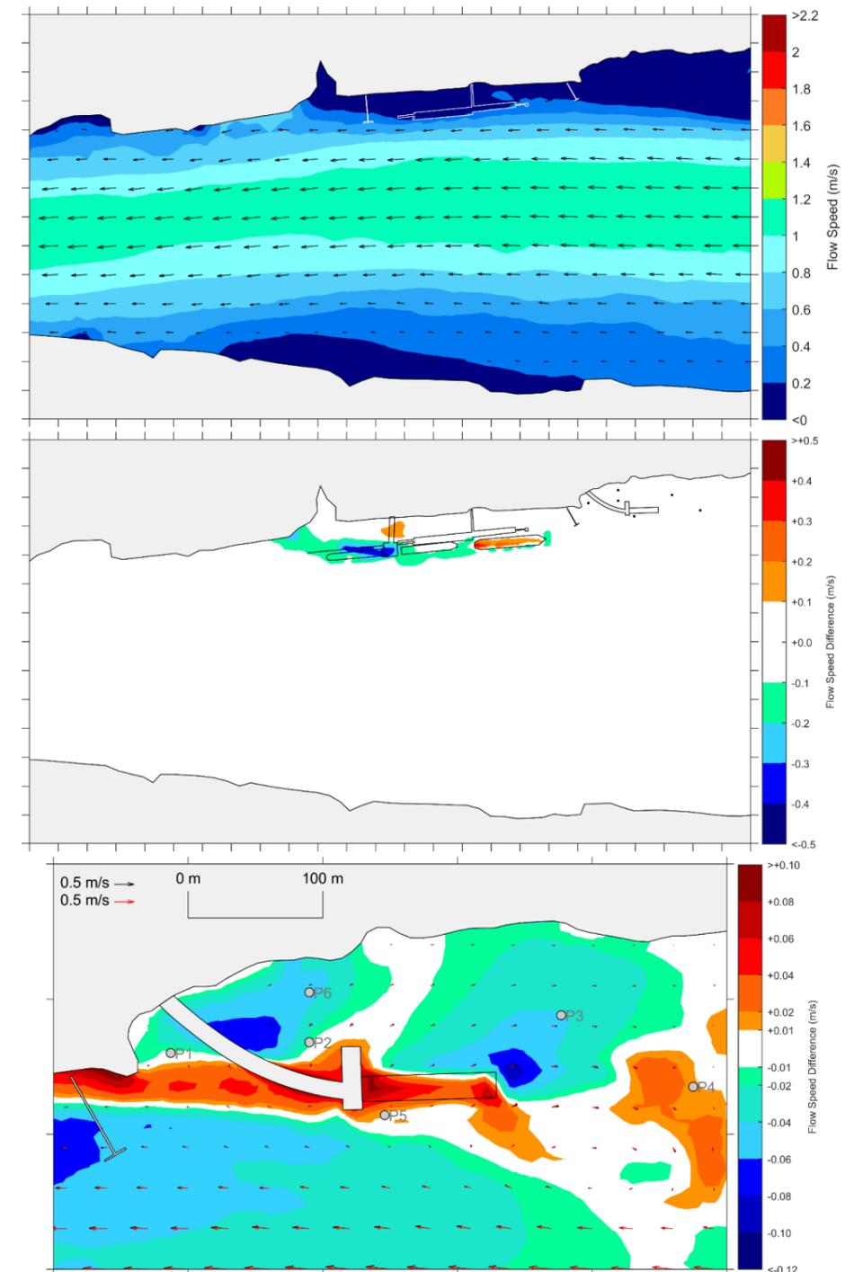
Figure 3.12: Baseline flows speeds during flood tide (top). Effect of Cumulative scenario on baseline flows (middle and bottom).
