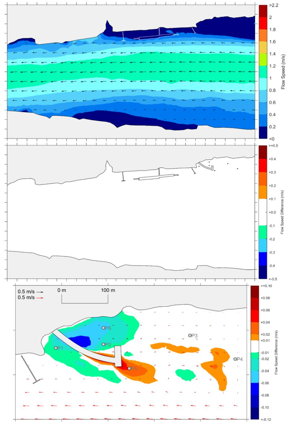
Figure 3.1: Baseline flow speeds during flood tide (top). Effect of AIL Facility (middle and bottom).
