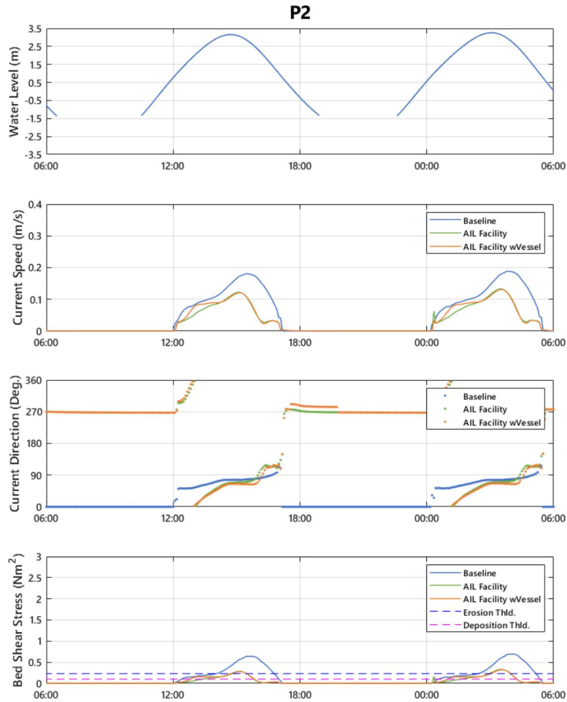
Figure 3.4: Comparison of current speed, direction and BSS as a result of the AIL Facility and AIL Facility with RoRo vessel compared to the baseline at P2.
