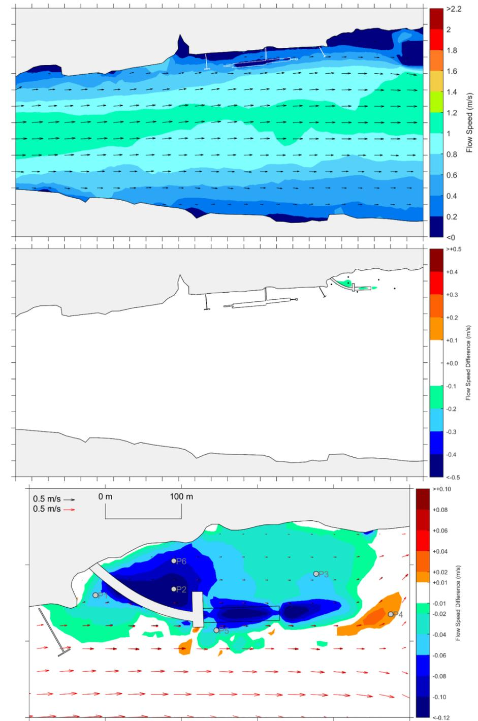
Figure 3.9: Baseline flow speed during ebb tide (top). Effect of AIL Facility with RoRo vessel on baseline flows (middle and bottom).
