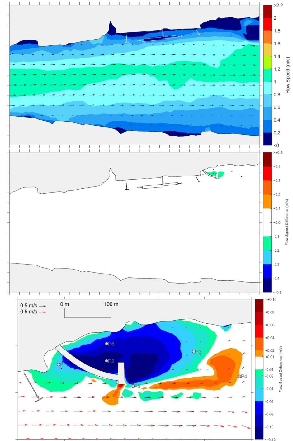
Figure 3.2: Baseline flow speeds during ebb tide (top). Effect of AIL Facility (middle and bottom).
