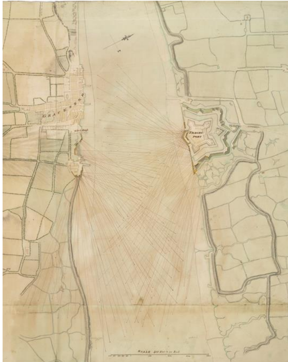
Plate 7: Detailed extract from a drawing by Thomas Hyde Page in 1778, showing proposed works at Tilbury and Gravesend Forts and the lines of fire
