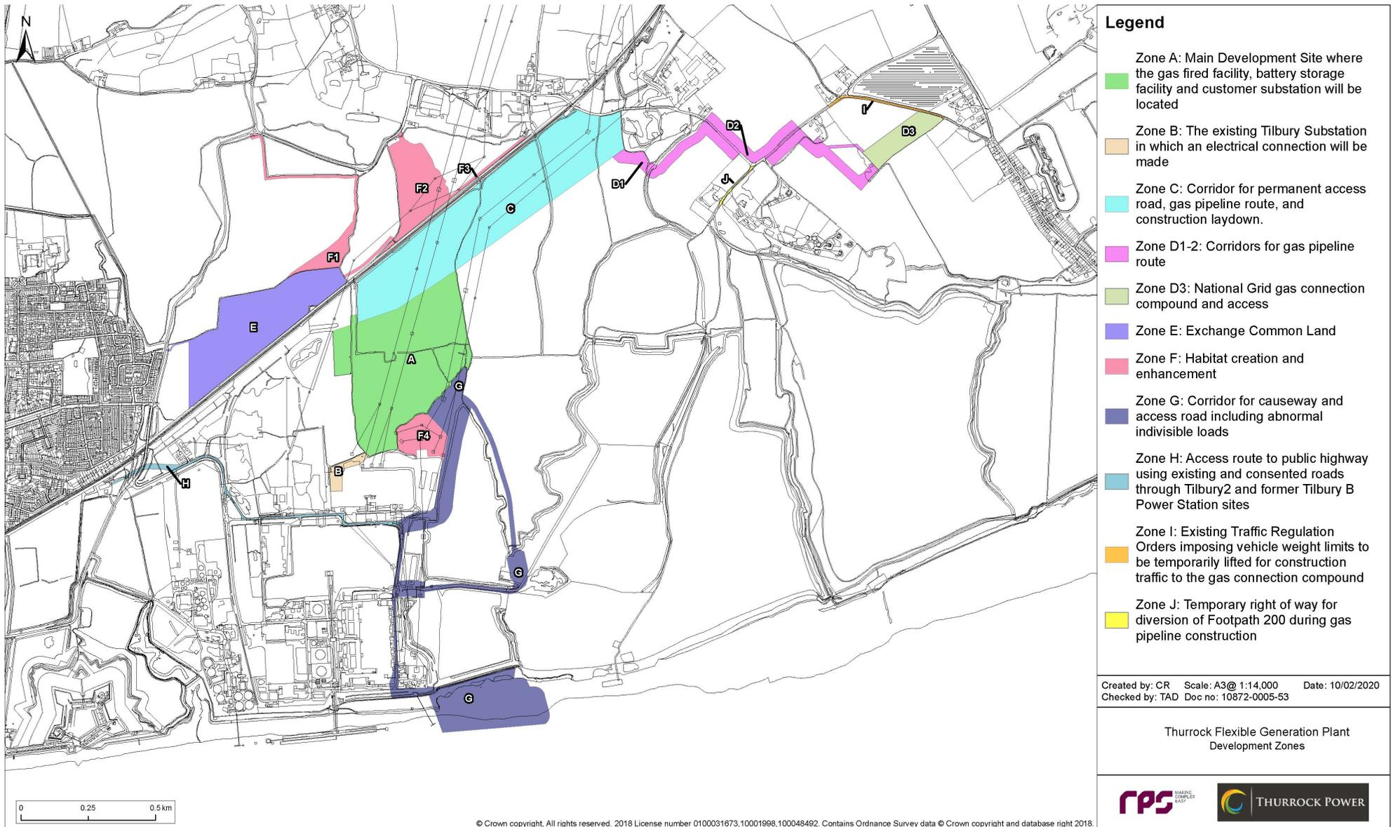
Figure 2: Thurrock Flexible Generation Plant Development Zones. All works outlined here relate only to the Main Development Site (A) (modified from RPS, 2019)
