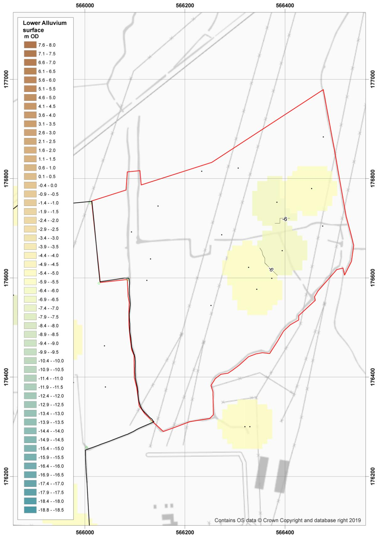
Figure 9: Surface of the Lower Alluvium (m OD)
