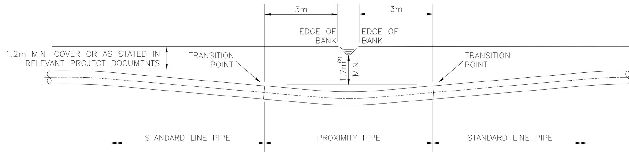
FIGURE 1: MINOR DITCH OR STREAM CROSSING
