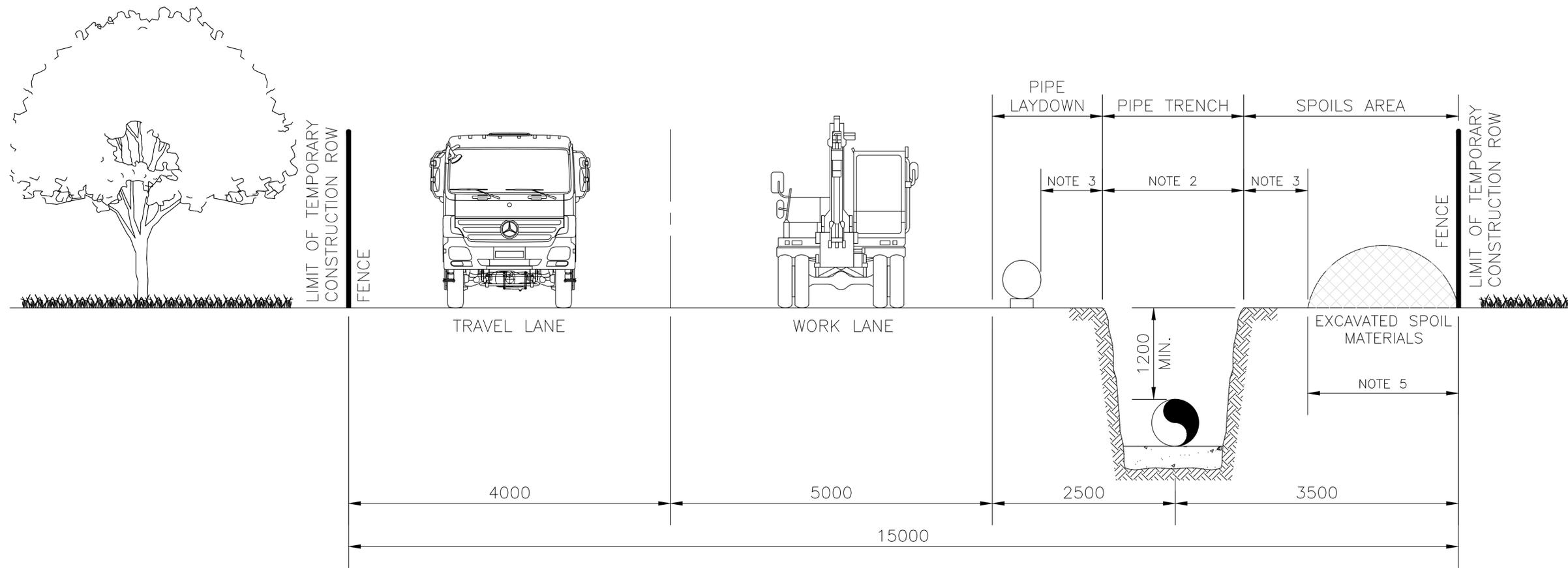
FIGURE 1: TYPICAL TEMPORARY PIPELINE CONSTRUCTION RIGHT-OF-WAY
