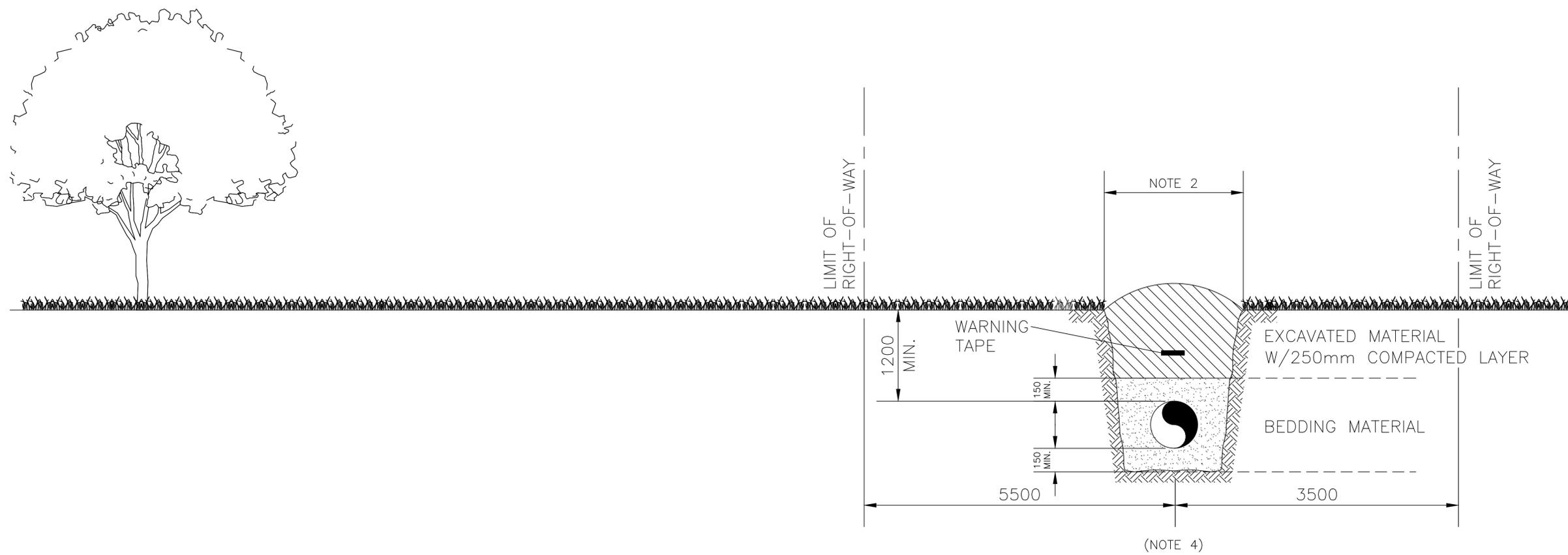
FIGURE 2: PERMANENT GAS PIPELINE RIGHT-OF-WAY (R.O.W.)
