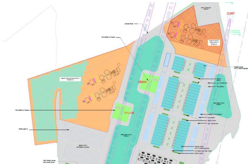
Figure 4: Indicative carbon capture layout
